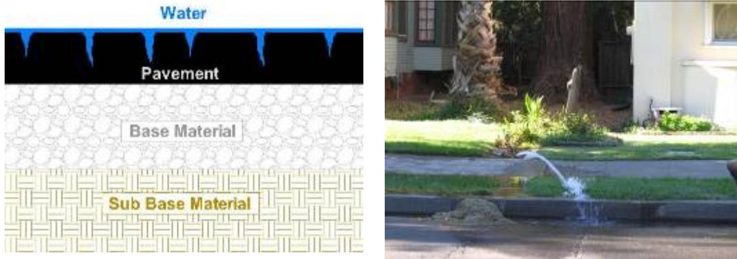
**Figure 4:** **Left** - Water penetrates the pavement and into the base via cracks in the asphalt.
